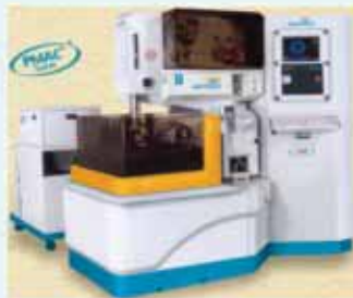
2. CNC Wire-EDM Machine with inclined surface machining capability (Model: SprintCut WIN from EMTL Pune): Procured and installed
