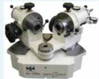
3. Computerized Double Flank Gear Roll Tester (Model: DO 125 K PC): Procured and installed
