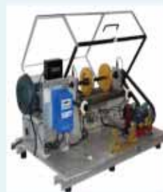
6. Machinery Fault Simulator (Model: MFS 2010 PK-7 from Spectraquest Inc. USA): Procured and installed
