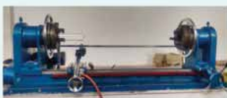
Double Chuck Lathe - Bore 70mm
